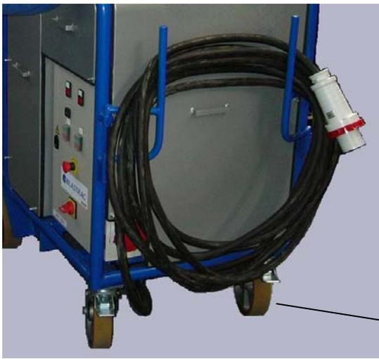
The dustcollector is equipped with a cable support. Wrap the supply cable over it in order to avoid damaging during transport.
