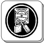
Prior to any repair works on the dust collector and its drives, secure the dust collector against unintentional switching-on. Pull out the mains plug in order to do this. Also make sure there is no air pressure on the pulse system.
