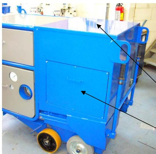
Remove the upper cover and side door to access the filter cartridges and lifting frame.
