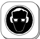
**All persons in the proximity of the dust collector must wear ear protectors, safety glasses with lateral protection as well as safety shoes. The operator is obliged to wear close-fitting protective clothing.**
