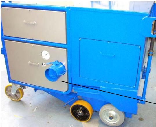
Remove the dust hose connectors in order not to loose them and to avoid damage to the machine and parts.
