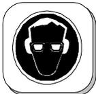
All persons in the proximity of the dust collector, when it is working, must wear safety glasses with lateral protection and safety shoes. The operator is obliged to wear close-fitting protective clothing.
